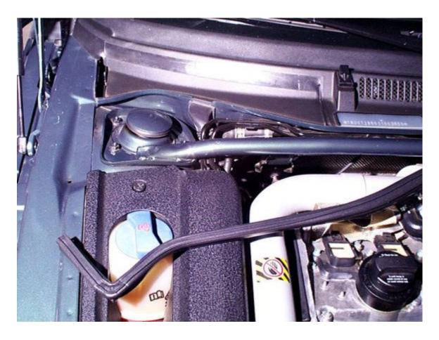
At the letf corner of the windshield, where the plastic pieces is, lift up at that corner. Pull back this piece. It's stuck in a grove below the glass.
