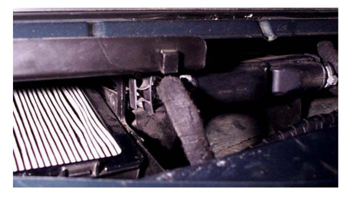
The connectors come off the ECU easily then push them out of the way to remove the ECU.,dt> Reve
